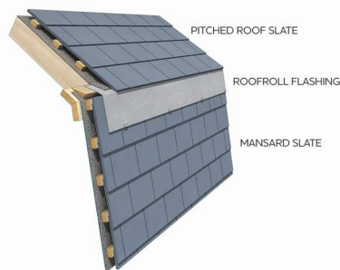
MANSARD SLATE ROOF DETAIL WITH FLASHING
