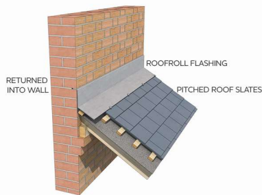
LEAN-TO SLATE ROOF ABUTMENT DETAIL
