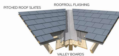
SLATE ROOF VALLEY DETAIL
