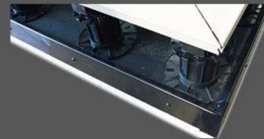
Pedestals running along an edge of an elevated area (flat roof, balcony or terrace) have edges that can be broken off to create straight edges
