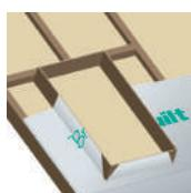
**4.3** Fold the flaps back up to the sides of the window and staple in place. Proceed with the next layer ensuring to follow the horizontal jointing detail.
