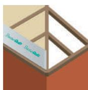
**8.1** Install the BreatherQuilt over the rafters, cutting the product to sit on the hip on the roof, and staple in place.
