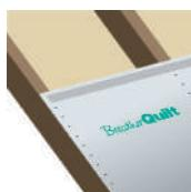
**2.1** Start at the bottom of the roof by rolling BreatherQuilt across the rafters and staple in place. BreatherQuilt features an easy to use built in tape with easy peel backing
