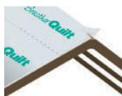
**6.1** Roll out the BreatherQuilt and fix in place using staples. Cut along the centre of the ridge beam and staple to the ridge beam to secure.
