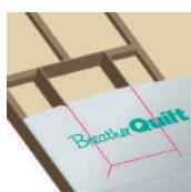
**4.1** Lay the BreatherQuilt over the window and cut out the section within the frame of the window (as detailed in drawing) on the top layer of BreatherQuilt only and fold this back.
