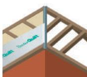
**7.1** Install the BreatherQuilt over the rafters, allowing the edge to drape over the valley gutter. Staple the product to the rafters, leaving the section over the valley loose.
