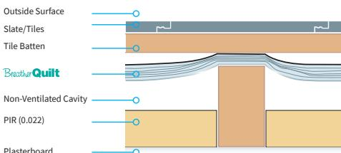
**U-Value table** New Build (0.13) calculations are based on 47mm wide rafters. Refurb (0.18) based on 50mm wide rafters. All calculations include the effect of cold bridging.
