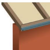
**3.1** Install a suitable eaves carrier over the rafters so that it runs down into the gutter (to manufacturers guidelines)
