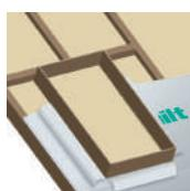
**4.2** Carefully cut and remove the rest of the material around the window's edge.
