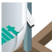
**7.2** Pull back the breather membrane on the product and carefully cut away the rest of the insulation, leaving just the grey membrane in the valley.
