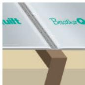
**1.3** Using the YBS BreatherQuilt 75mm Waterproof Tape, tape over the joint and ensure it is fully sealed.
