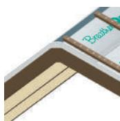
**6.2** On the other side of the roof, roll out the BreatherQuilt and butt-joint to the first piece. Using the YBS BreatherQuilt 75mm Waterproof Tape, tape over the joint and ensure it's fully sealed.
