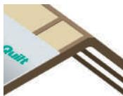
**5.1** Install the BreatherQuilt on both sides of the roof.
